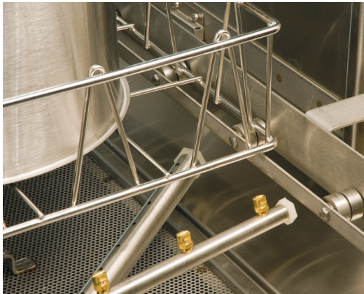
Rollers make getting large racks in and out of the pot washer easier.
