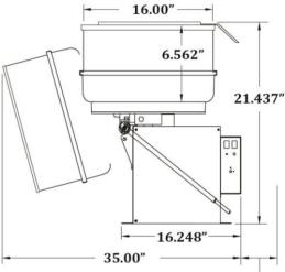
6" Recommended Min. Clearance between wall and Cntl Box for Service.
