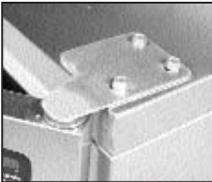
**HEAVY-DUTY 1" STAINLESS STEEL TUBULAR HINGE...** Full length eliminates torque on top hinge. Mounted with 1" bushing and 12 gauge stainless steel mounting bracket. Keeps doors properly aligned and withstands rugged use.
