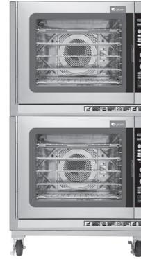
A high efficiency gas combustion chamber heats the cooking cavity in steam, combo and oven modes. All condensate exits through cavity drain. Oven/steam vent is provided. Safety or low water cutoff provided and reservoirs automatically drain when unit is turned off. Standing pilot with electronic ignition is standard.
