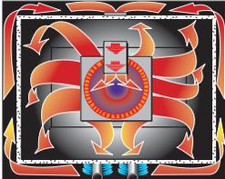
Turbo-Flow System provides even temperatures throughout the oven cavity.
